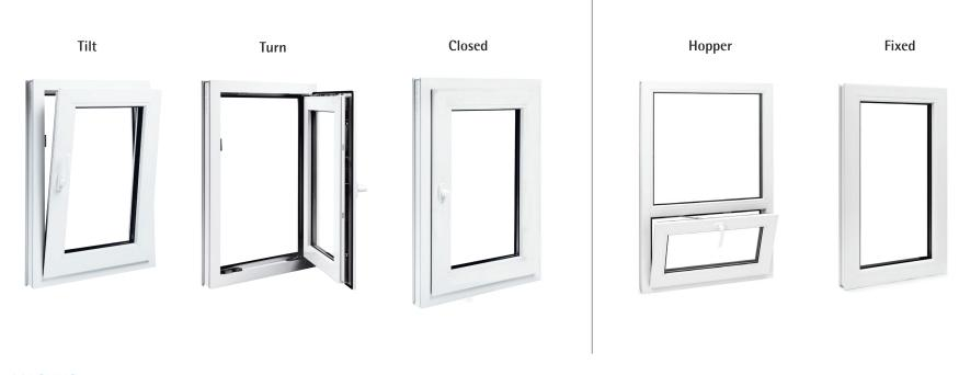
MAGNUS 4500 tilt-turn window is unique and versatile with its three-windows-in-one design: A secure top-venting hopper in the tilt position, an inward opening casement in the turn position and a tightly sealed picture window when closed.
